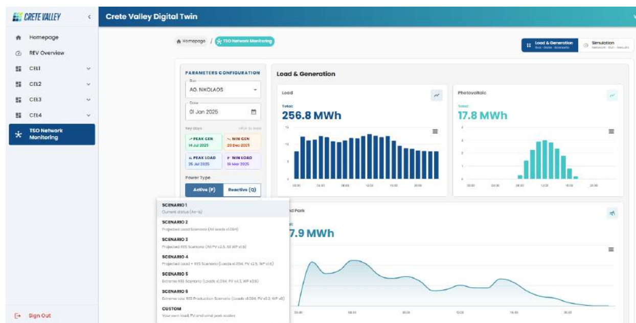
Figure 49: TSO data analytics interface for scenario-based visualization of hourly substation load and generation profiles
